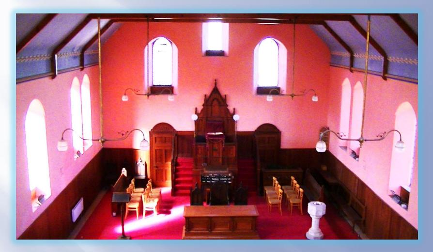
Church finished and cleaned. The red matting on the choir area and aisles was turned upside down to reveal fresh new colour! Paintwork was re-done where necessary using specially mixed paints to match the existing colours as nearly as could be managed. The window heaters were taken down and rewired, the wall heaters were repainted with radiator enamel and all the electrics were checked for safety. Missing slates were replaced outside and a bit of pointing done.
